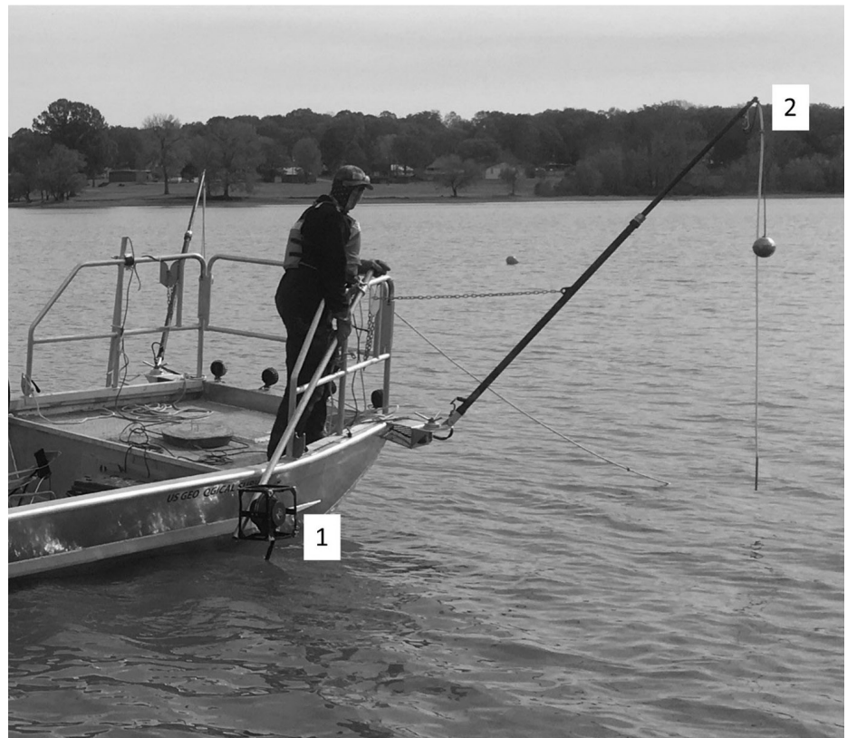
Figure 1. Drive boat used to deploy a dual-deterrent (acoustic deterrent and electricity) fish herding technique (method similar to Ridgway et al. 2021) to clear fish out of the navigation lock at Starved Rock Lock and Dam (Illinois River, LaSalle County, Illinois, USA; 41.324670°; -88.986316°). 1: The starboard speaker (LL916C, Lubell Labs, Columbus, Ohio, USA), 2: the starboard anode configuration composed of one stainless-steel sphere (6.4 cm diameter) and one stainless-steel cable (2.2 m length insulated cable with 20.3 cm uninsulated section at the end) (photo Josey Ridgway – U.S. Geological Survey, used with permission).
