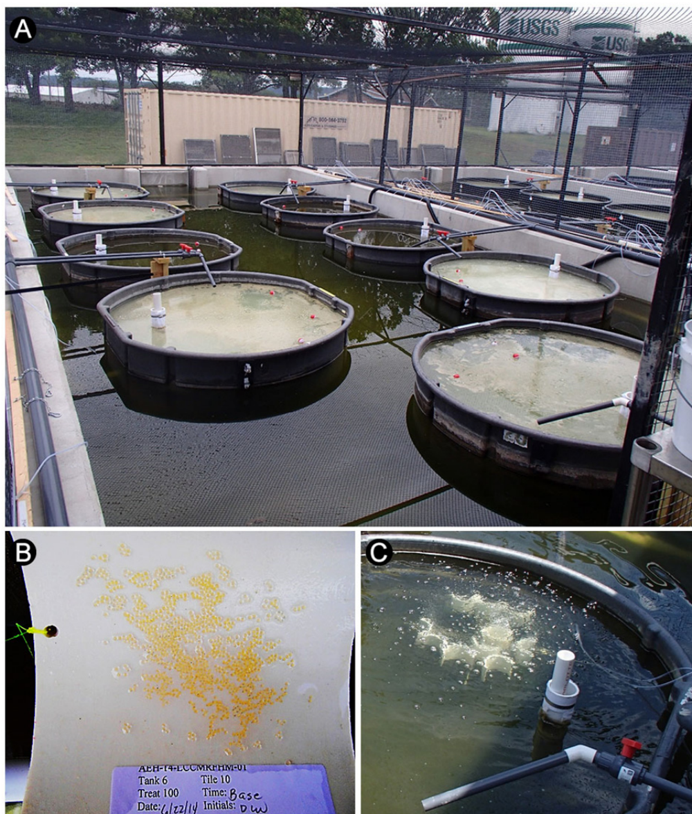
Figure 1. Test system. A) Mesocosm test system consisting of nine independently plumbed 1000-L tanks within each of four 0.004-ha concrete ponds. Water was supplied to test tanks from a 0.25-ha earthen pond. Concrete ponds were filled with water and covered with shade cloth to moderate diurnal temperature fluctuation. B) Spawning substrates with newly deposited eggs on the concave surface. A digital photograph was taken of substrates for enumeration of newly deposited and eyed-eggs. C) Incubation of spawning substrates in the test tank atop a bubble wand. Photographs by D. Waller.
