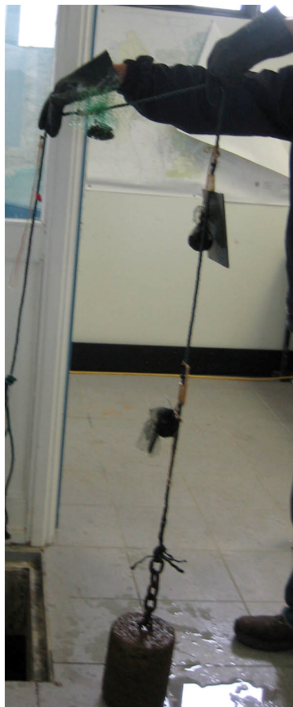
Figure 3. Bags with adult mussels and PVC juvenile settlement plates attached to the suspension rope, deployed in the drinking water treatment plant chambers (photograph by Sara Meehan).
